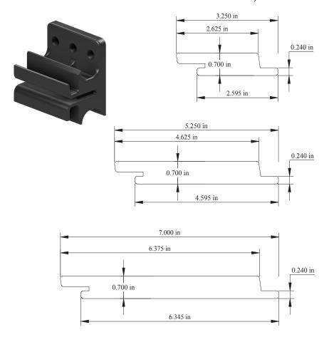
3/4" Air Gap Structural Sheath Framing Stud
