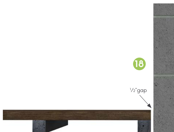
Gap between boards and solid surfaces
