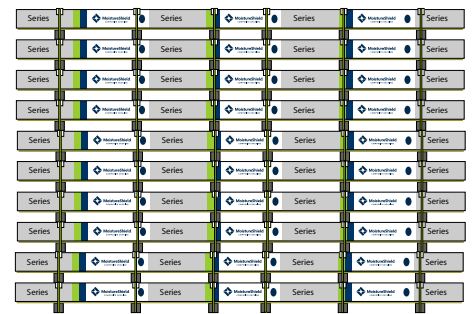
Stable Stack of Decking Units
