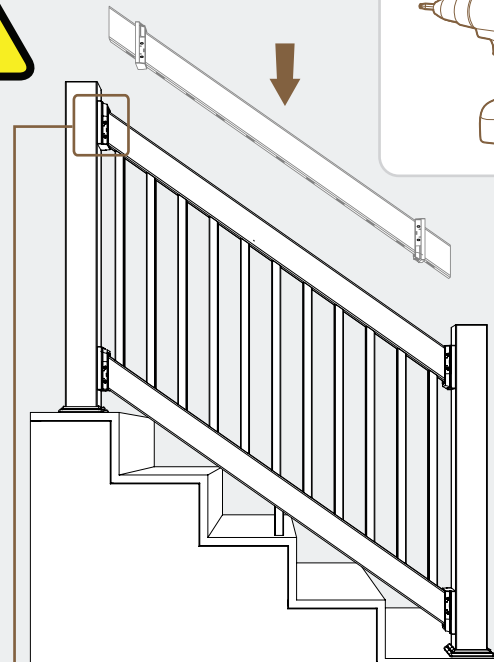
FIG 1 Long leg of P-Shaped Aluminum Stiffener needs to face towards inside of deck.
