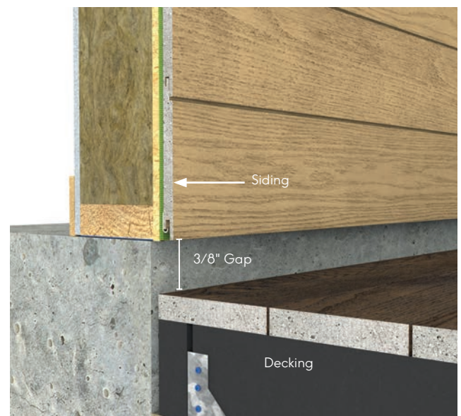
Fig. 7 - Install detail above deck
