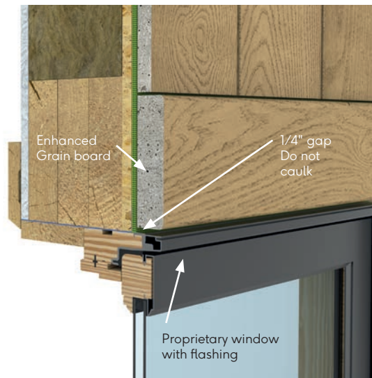
Fig. 25 - Window head with Enhanced Grain
