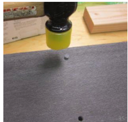
Tap plug 'flush' using a PLASTIC Mallet.
